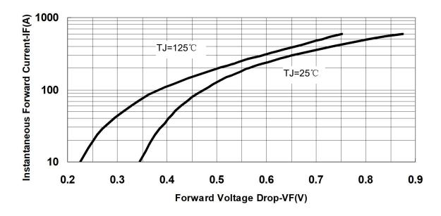
Fig.3-Typical Instantaneous Forward Voltage Characteristics
